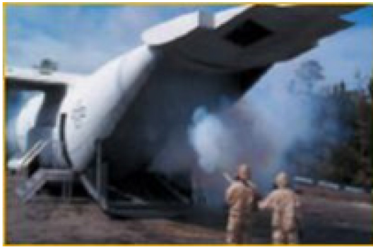
Figure 3-26: Aircraft Decontamination by GD5 with Decofogger System. ( www.oshodefence.com , www.militarysystems-tech.com ).
