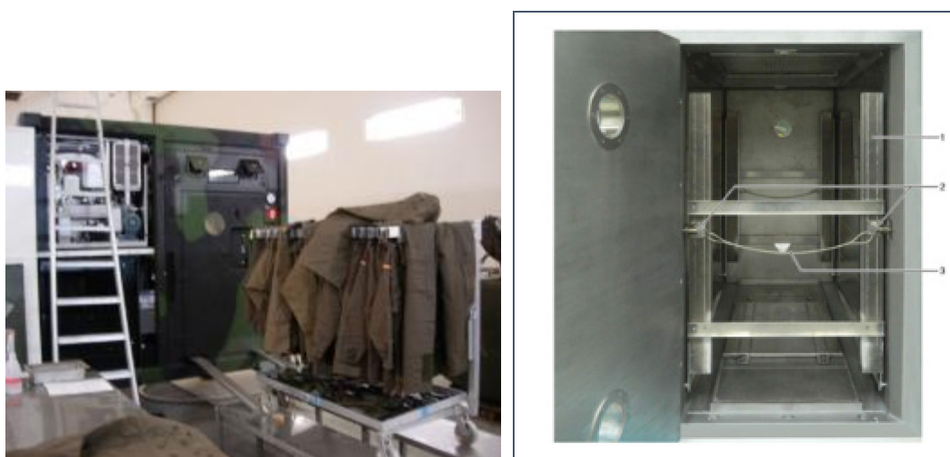
Figure 3-10: Hot Gas / Steam Chamber (WIS).
