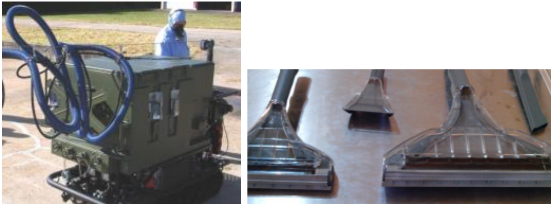
Figure 3-12: The Fielded Spray-Extraction System, WIS.
