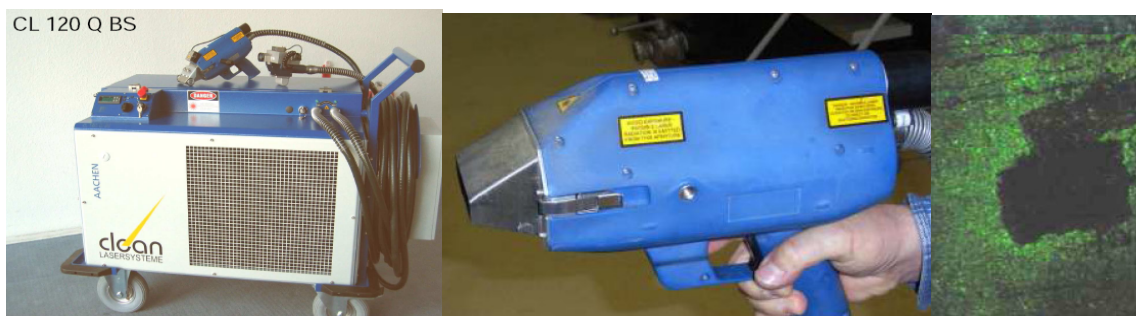
Figure 3-24: Clean Laser System, Manual Application of Laser Radiation on Surfaces (WIS).
