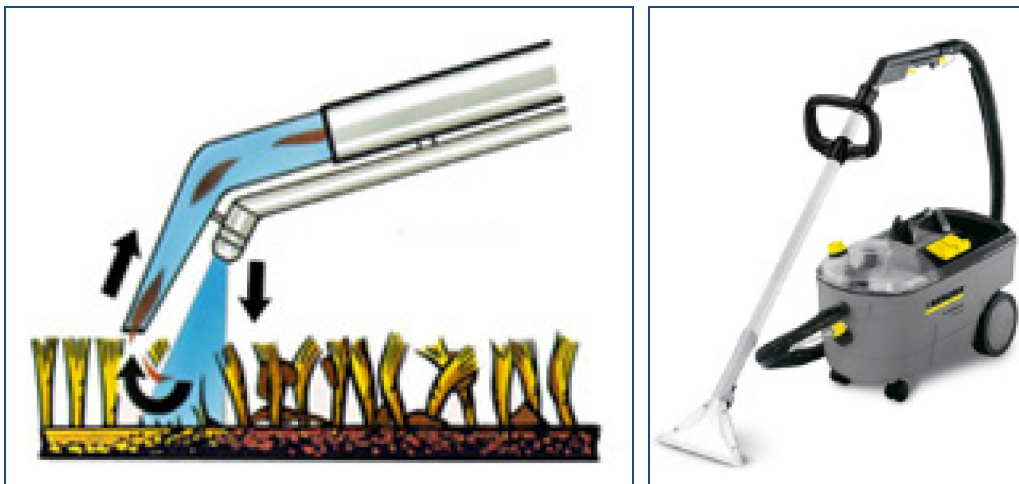
Figure 3-11: Operational Principle of a Spray-Extraction Device (Left), Civilian System (Right) ( www.karcher.com ).
