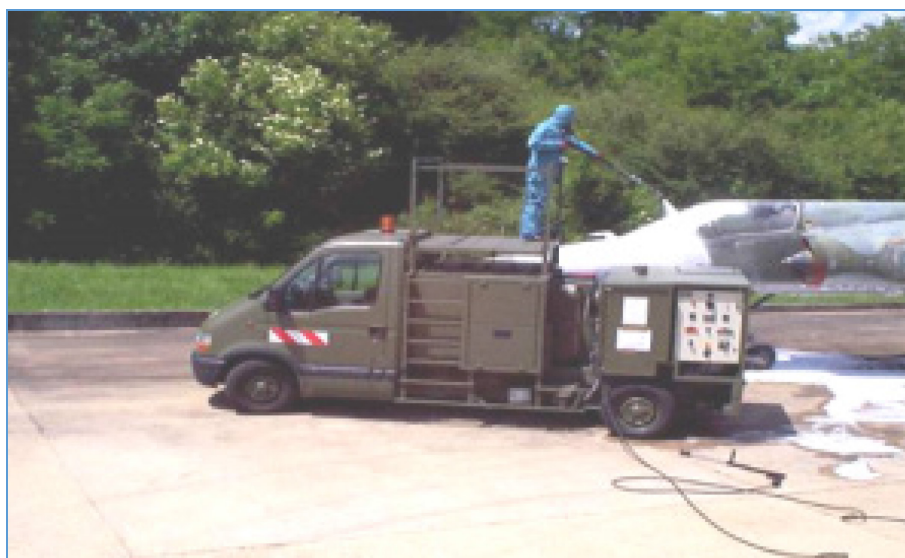
Figure 3-25: Aircraft Decontamination with French Q2000 Decontamination Solution and SYMODA Dispenser (DGA CBRN Defence).
